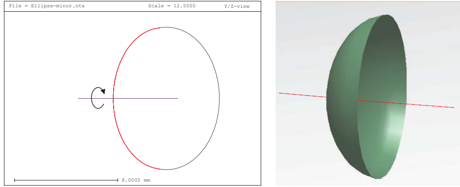
Figure 8.6: Definition of an elliptical section at the minor axis ( K > 0 ). Left: Section of the ellipse. Right: Perspective view showing the resulting surface.
